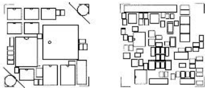
Fig. 8: The SLC multi-layer printed circuit board with dimensions of approx. 44x44mm (1.8 by 1.8 inch)
